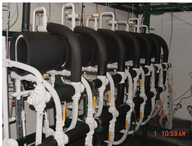
Figure 2. Picture of test section which was comprised of 14 heat exchangers.
